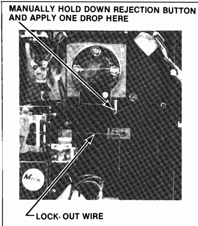
Figure 3-6 Close-Up View of Lubrication Point
