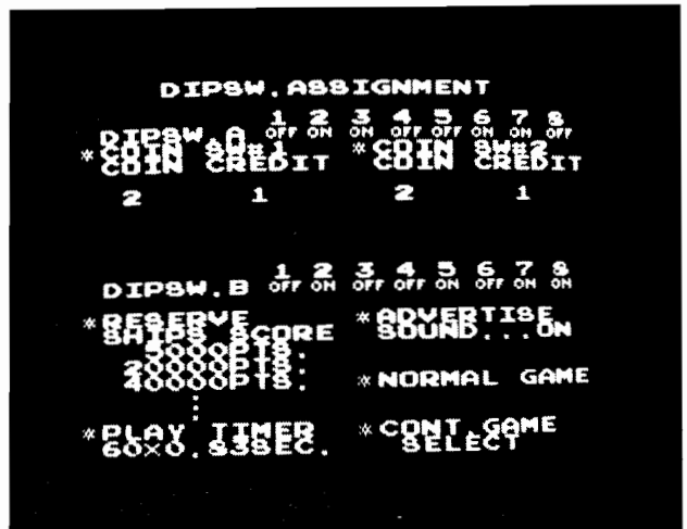
Self-Test - Dip Switch Assignment
