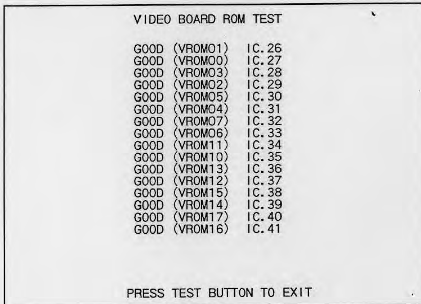
FIG. 3.1d MEMORY TEST (VIDEO BOARD ROM TEST)
