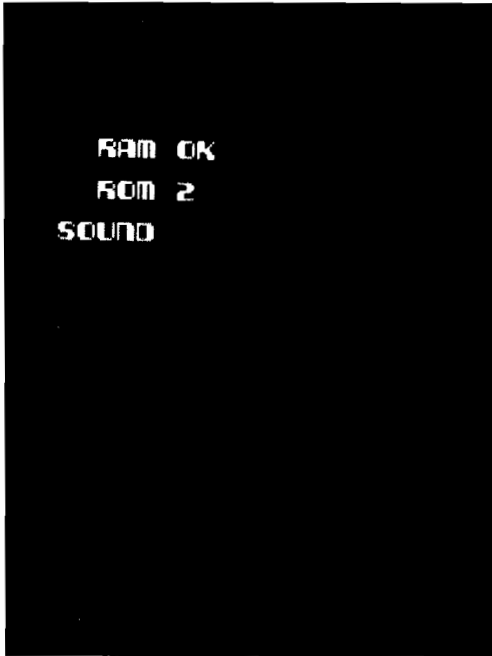
Figure 2-3 Self-Test Display (ROM Failure)
