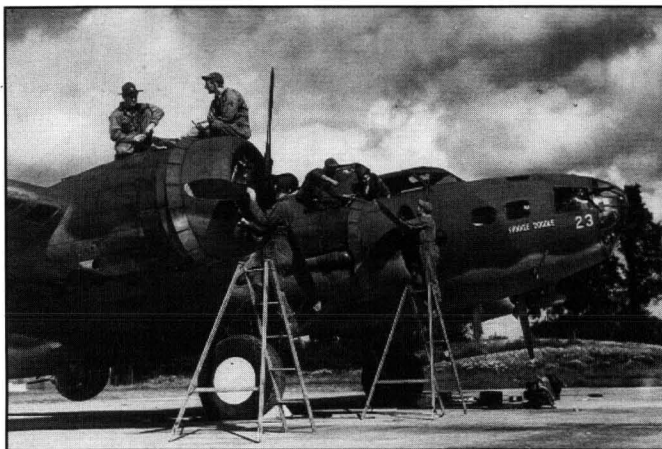
Ground crew giving a complete and careful overhaul to a B-17F after a non-combat flight. On the ground below the nose is the portable generator known as the 'putt-putt'.
