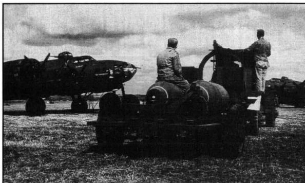
Bomb service truck and trailer approach a flight of B-17's with 2 one-ton bombs. Exploding fragments from these bombs could travel over a mile in distance.
