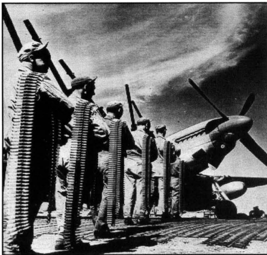
Armorsmen each carrying one 0.50 calibre machine gun and a belt of ammo prepare a P-51 Mustang for an escort mission.
