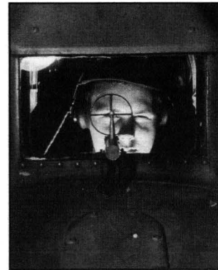
The tail gunner off a Flying Fortress aims through the ring-and-bead type gunsight.
