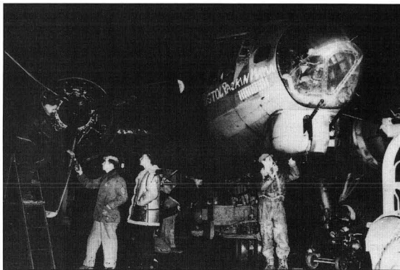
"Pistol Packin' Mama" is readied during the night for a dawn take off. Bombs are loaded, guns and engines checked. The ground crew chief is on the ladder (left).
