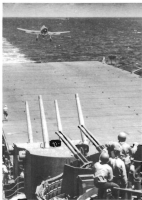
A U.S. Navy fighter gets ready to land. Note the arresting wires on the flight deck. Courtesy of the U.S. Navy
