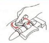
The best adjustment may allow you to see only three marks, or four slightly blurred marks. When you have completed the IPD adjustment, proceed with the FOCUS adjustment.
