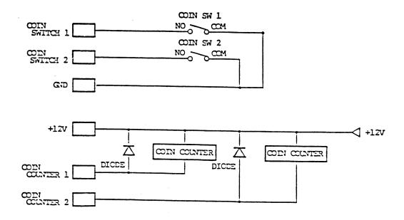
FIGURE 3 - Coin Counter/Coin Switch Circuit
