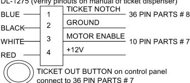
When connecting ticket dispenser, check manual of ticket dispenser. Colors may be different from above diagram. Thickness, width, and paper quality of ticket can affect accurate counting. Crumpled and used tickets cannot be used.
