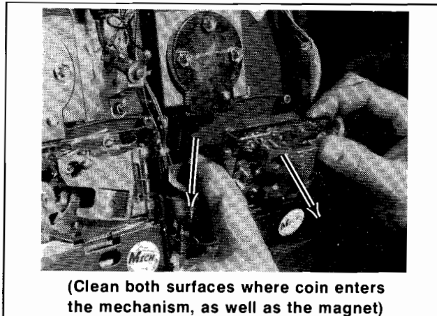
Figure 3-3 Removal of Coin Mechanism
