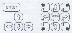
Numbers 1, 3, 7, and 9 take the cursor directly to the corners of the display; use the even-numbered keys for finer navigation.
