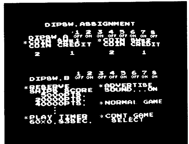
Self-Test - Dip Switch Assignment
