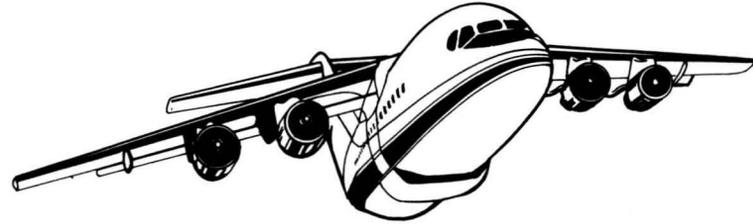
with its provision of passenger comfort in a small aircraft. As well as the noise levels being low, it is one of the widest of the single-aisle aircraft and, since the wings are attached to the top of the fuselage, it offers unrestricted views out of the windows. The 146-100 seats 82-93 passengers six-abreast and the -200 typically 96 but as many as 109, also six-abreast. The -300 enters new realms of comfort seating 100, but only five abreast.
