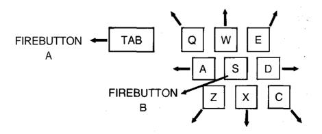
These keys perform the same functions as the numeric keypad. The arrows indicate equivalent joystick movements when using a second joystick on the PCjr.
