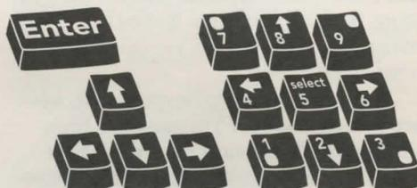
Numbers 1, 3, 7, and 9 move the cursor directly to the corners of the display; use the even-numbered keys for finer control.
