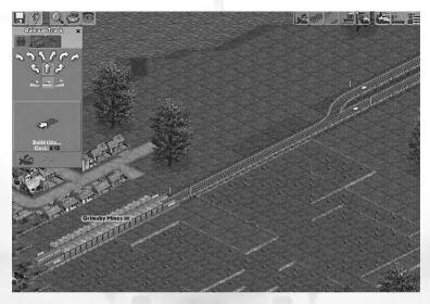
This layout is a simple double-track line connecting two stations, one at either end of the line. The two tracks in the double-track section run in opposite directions, and each has single-direction signals facing in the direction of travel placed at regular intervals along the way. As is true in the previous example, signals should be spaced no shorter than your longest train.
