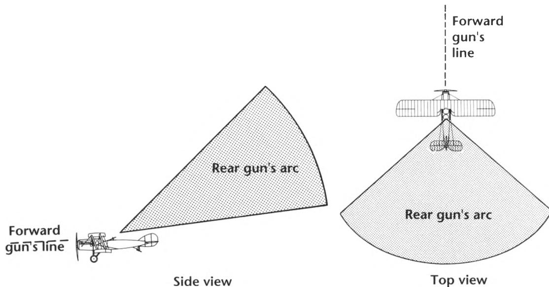
■ The F.E.2b has a unique gun configuration. The gunner can operate two separate machine guns. Both are mounted on a swivel. The rear gun has a limited arc, as its line of fire must clear the top wing of the F.E.2b. This results in a large vulnerable area directly behind the aircraft.
