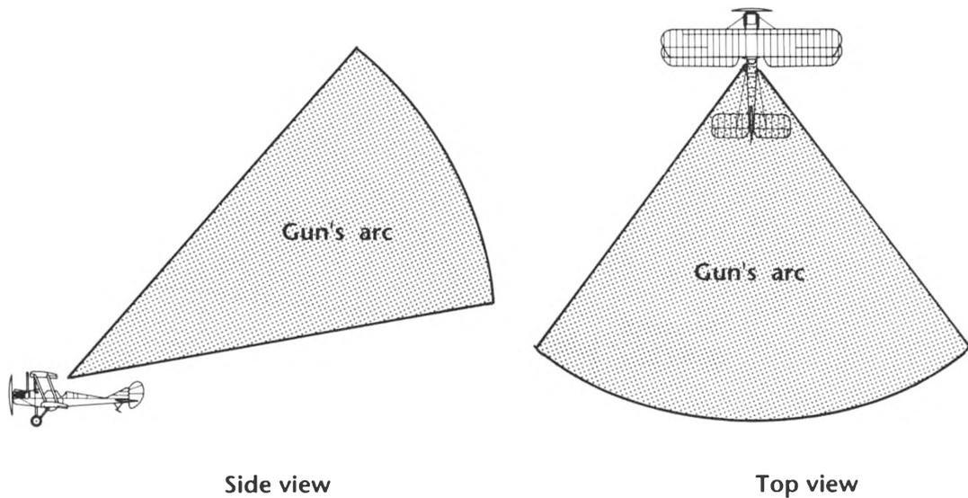
■ On these aircraft, the rear gun was mounted on a swivel, whereas the forward-firing gun was fixed. The standard attack tactic against two-seaters was to approach from its blind spot—from behind and below the two-seater.
