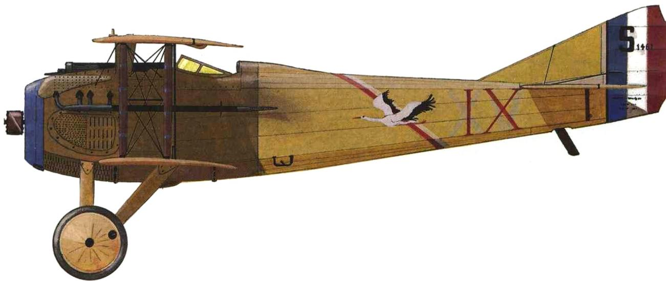
When the Spad 7 entered service in 1916, it quickly earned a reputation for being both rugged and durable. Spad pilots could out-dive any of their adversaries, though they could not turn as quickly as most German scouts.
