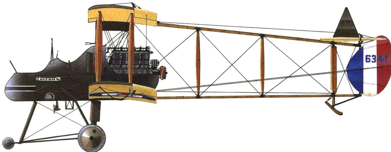
The "Fee" was an ungainly two-seat aircraft. The propeller was located behind the pilot.
