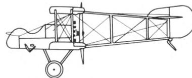
The D.H.2 was a nimble, highly maneuverable bi-plane that helped end the Fokker Scourge in 1916. It was one of the earliest fighters to have an engine mounted behind the pilot in a pusher-type design. Unfortunately, the engine was totally unreliable, and often several D.H.2s out of each patrol would have to abort because of engine trouble. Nevertheless, it served well into 1917. By this time, however, the D.H.2 was hopelessly outclassed by the newer German aircraft.
