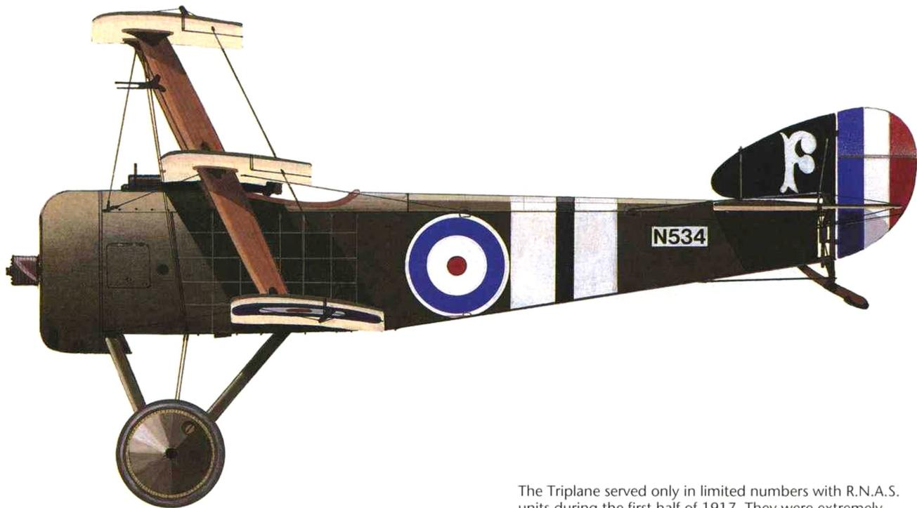
The Triplane served only in limited numbers with R.N.A.S. units during the first half of 1917. They were extremely nimble, but underpowered, aircraft.
