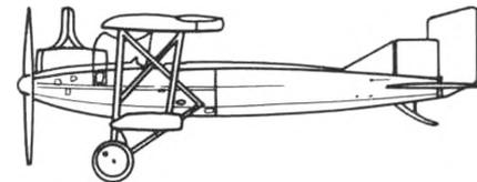
The Junkers J.I was a two-seat attack bomber used by the Schlstaffeln (ground attack squadrons) throughout 1918. The vital areas of the plane were covered with armor plating, making it a very difficult aircraft to shoot down. It carried two forward-firing Spandau's and one Parabellum for the gunner as its main armament. Unfortunately, it was an extremely heavy aircraft. This greatly impaired its maneuverability and general handling characteristics.
