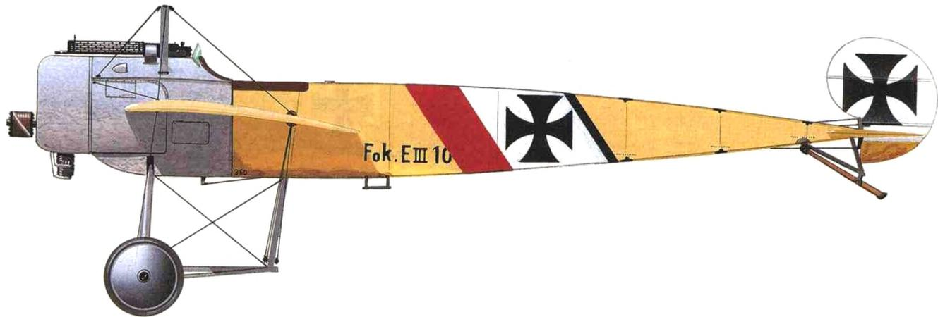
This particular Eindecker was flown by Ernst Udet in March of 1916. The Eindecker was the first aircraft to mount synchronizer gear allowing the machine gun to fire safely through the propeller arc. The Fokker Scourge was a result of the E.III's superiority over the Allied scouts of the time.
