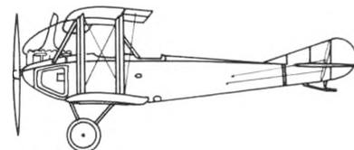
Appearing in early 1915, the Aviatik C.I served as a two-seat observation and artillery spotting aircraft. Like the B.E.2c, the gunner sat in front of the pilot. This arrangement restricted the arc of the gunner's machine gun, since the struts blocked his vision in certain directions. Slow and awkward in the air, it revealed itself to be highly vulnerable to fighter attacks. In 1916, an upgraded version appeared at the Front and was designated the C.III. It was only modestly successful.
