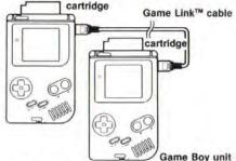
Connect the cable as shown in the diagram. After checking to make sure that the cartridges are properly set in place, turn on the power for both units. Press the SELECT button to select the play mode on ONE of the Game Boy® units. After the mode is selected, press the START button to begin play on both units. The unit which presses the START button will become the LIGHT TEAM on the LEFT side of the screen.
