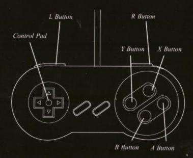
Control pad: ...... Controls all directional movement — left, right, up and down.
