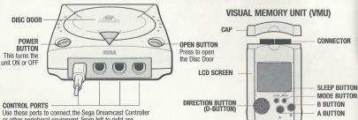
Use these ports to connect the Sega Dreamcast Controller or other peripheral equipment. From left to right are CONTROL PORT A, CONTROL PORT C, AND CONTROL PORT C, AND CONTROL PORT D. Use each port to connect controllers for players 1 to 4 respectively.
