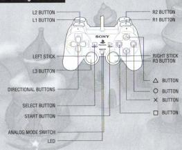
Note: The Left Stick of the DUALSHOCK™ analog controller is functional only in ANALOG mode when the ANALOG mode switch LED is ON (lit). Press the ANALOG mode switch to toggle the LED ON/OFF.
