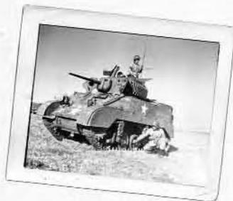
The 15-ton M5A1 "Stuart" light tank, introduced in early in 1943, has a 37mm gun fitted in the turret, a .30 caliber machine gun in the bow, a .30 caliber machine gun mounted coaxially with the 37mm cannon, and a .30 caliber machine gun on top of the turret. This light tank is fast and light and used primarily for scouting and reconnaissance missions. It is not designed to battle head-to-head with most German tanks.
